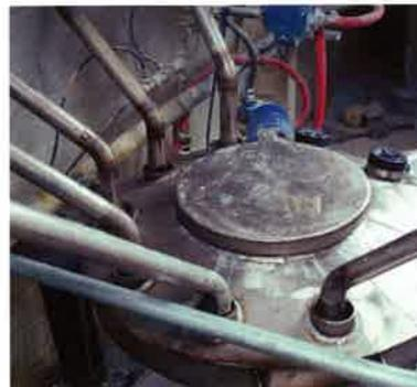
Neither the discharge pipe nor any of the six infeed lines touch the tank. No gaskets, no seals. Only air gaps. This eliminates vibration from the pumps and valves that control the liquid infeeds.
