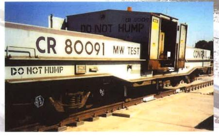
Testing the Ampacet rail scale. Hydraulic jacks extend down from the center 'doghouse' of ConRail's test car, lifting the car into the gir and concentrating 100,000 pounds certified weights on the scale.
