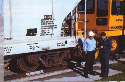
Process engineer Mark Wolfe (left) and Richard Bonine of Ampacet collect information off the side of the rail car. The yard engine, with Scott Taylor at the controls, is off the scale. The yard engine is periodically weighed as a rough check to make sure the scale remains calibrated.
